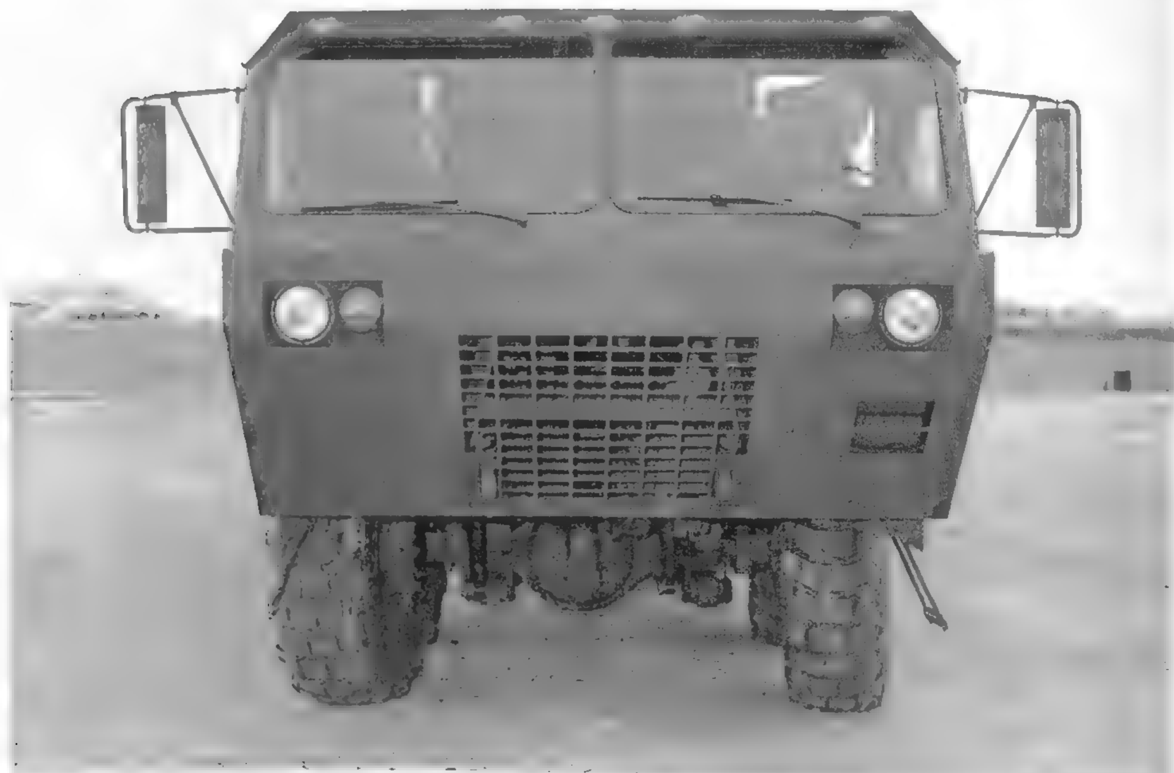
The backward rake of the lower portion of the cab gives the HEMTT a 43-degree angle of approach, which is important when operating off-road. (U.S. Army photo)
